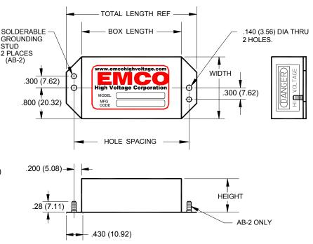
Dimensions are in Inches Dimensional Tolerances: ±0.03 (.76mm) (Metric Equivalents in Parenthesis)
